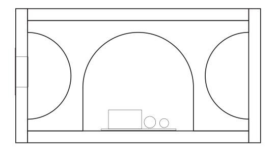
Side view of center brace C showing location of the crossover and binding post cup.
