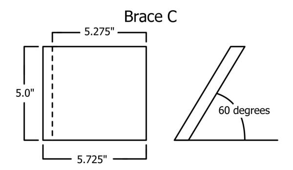
Measurements & placement for Brace C are not exact to allow for small differences in tolerance
